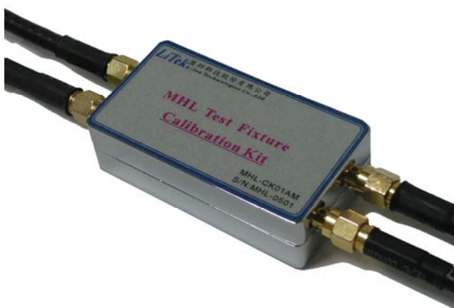
Fig2: MHL-CK01AM connected with SMA Coaxial cable form Equipment for calibration before testing.
